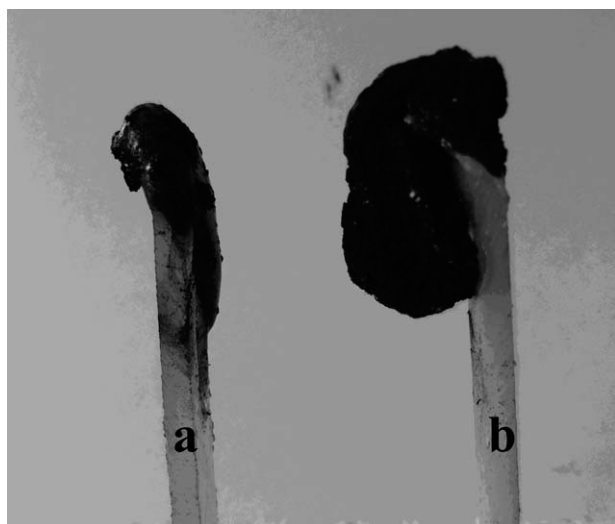
Figure 3 Char layer of the samples after LOI tests (a) pure PC, (b) PC/5 wt % HSOBA.
